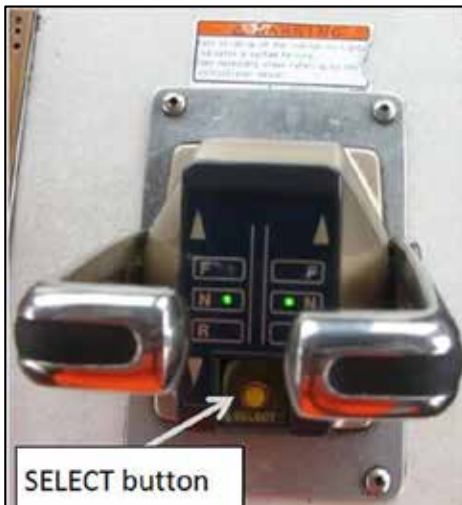
Figure 6. Hand levers on the C.7. Titan's propulsion control unit
