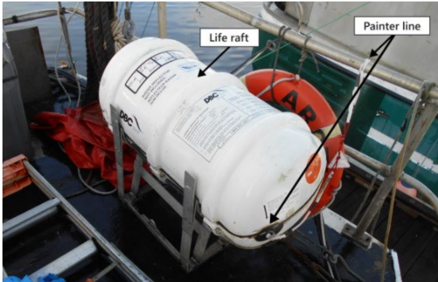
Figure 3. Stowage of the life raft on the Arctic Fox II (Source: Owner)
