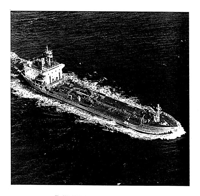
The M.V. "IRVING NORDIC" is an ice-strengthened product carrier designed to carry refined oil cargoes.
