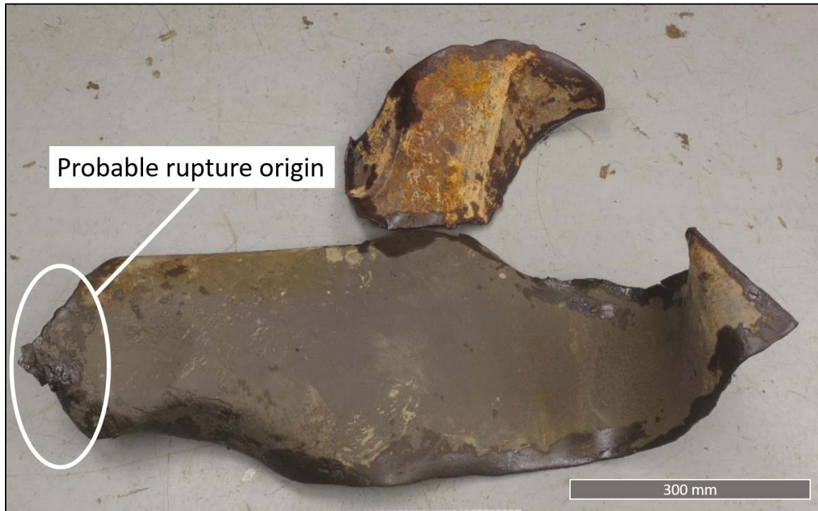
Figure 8. Ejected pieces of pipe (Source: Acuren Group Inc., with TSB annotations)
