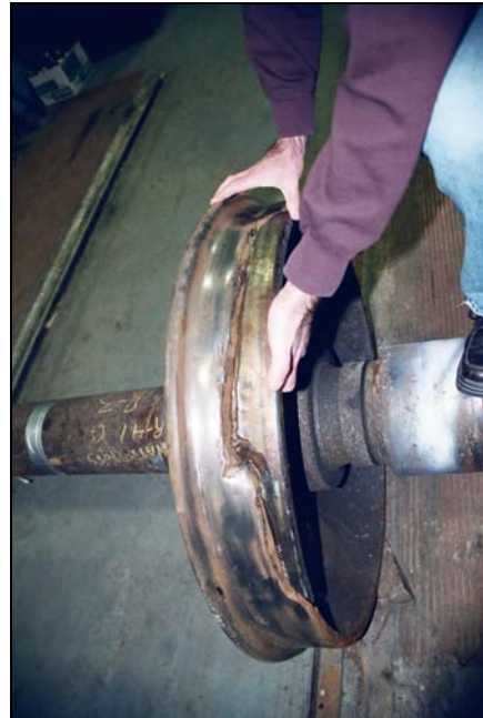
Photo 2. Broken wheel from car NATX 77085
