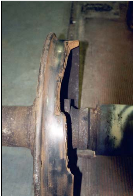
Photo 1. Matched rim section broken wheel
