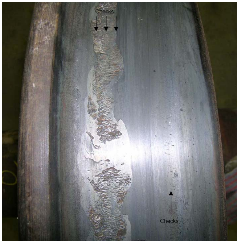
Photo 5. R3 wheel from car NATX 77085 – close-up of tread surface with two circumferential bands of heat checks
