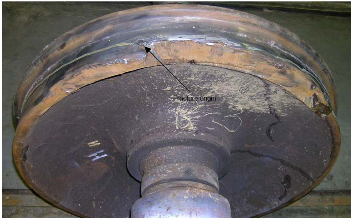
Photo 3. Broken R3 wheel from car NATX 77085
