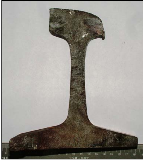
Photo 4a. Face de rupture C
