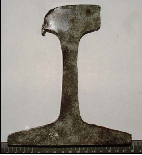
Photo 2a. Face de rupture A
