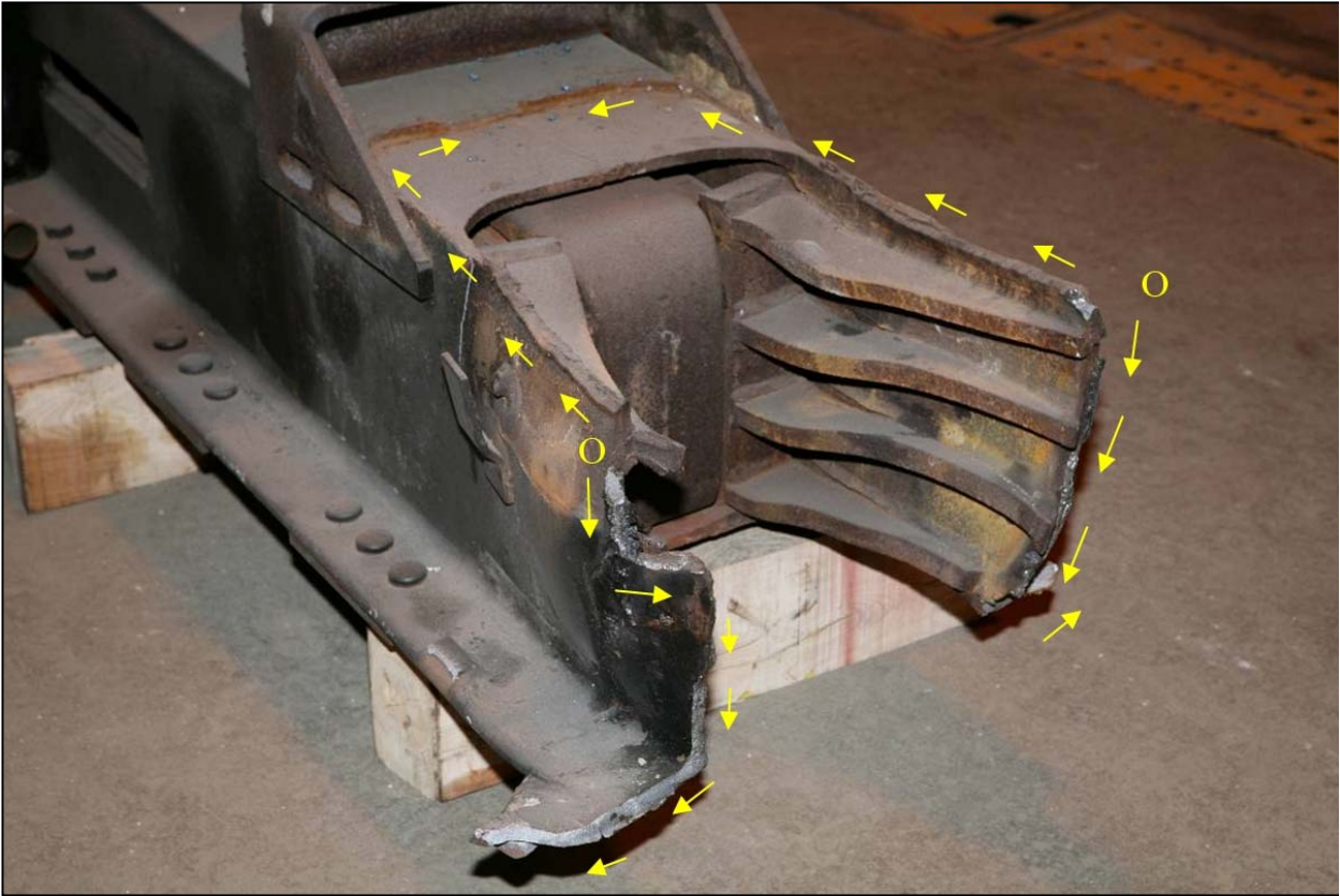
Photo 4. View of stub sill fracture, left side. Origin areas are indicated with “O” and the directions of crack propagation are indicated with arrows.
