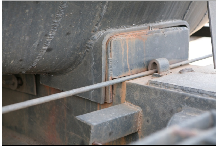
Photo 5. Bracket covering head brace
