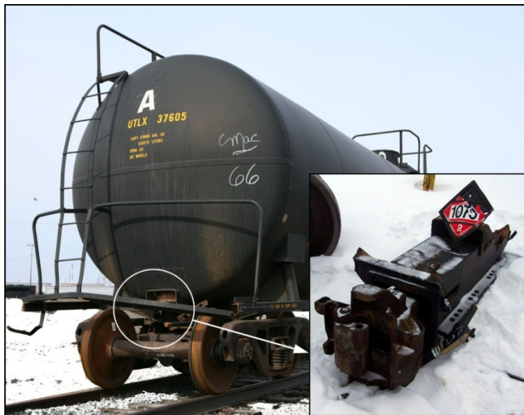
Photo 1. Car UTLX 37605 missing A-end stub sill
