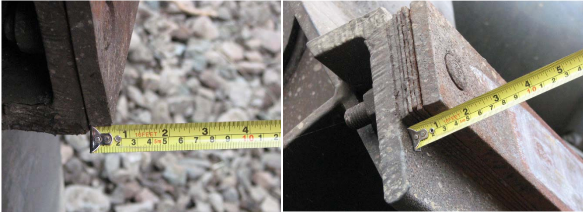
Photo 2. Body Side Bearings on B-end of car PROX 98433 (Left Photo - No shims at location BR; Right Photo - Approximately \frac{7}{8} inch shims at location BL).
