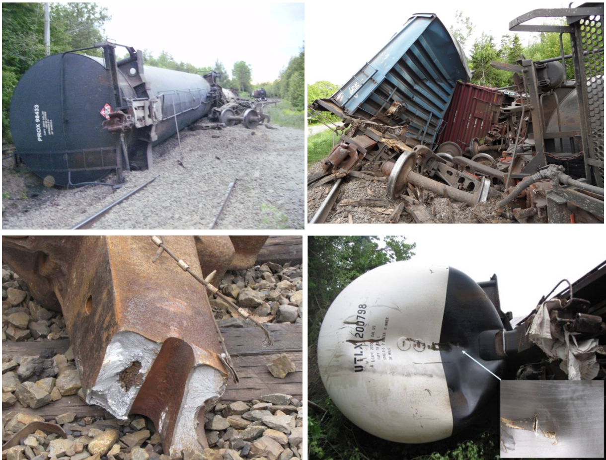
Photo 1. Derailed rail cars. Arrow bottom right (with inset) denotes location of head puncture on the residue hydrogen peroxide car.
