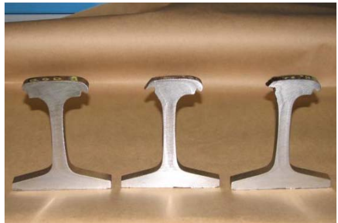
Photo 5. End view of sections of south rail in derailment curve.
