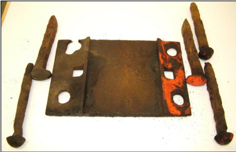
Photo 9. Older style tie plate and round track spikes
