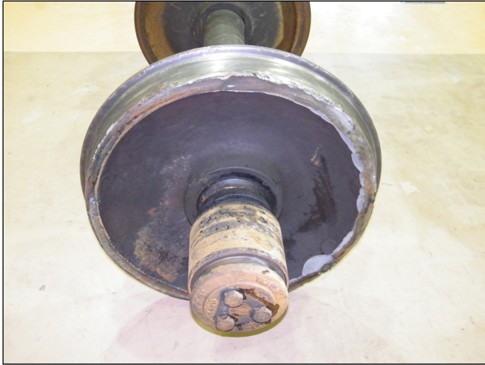
Photo 1. Wheel set with the broken wheel and mate wheel
