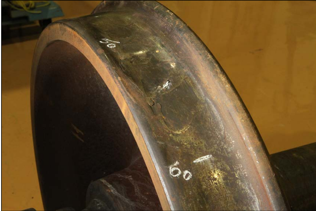
Photo 2. Typical slid flats on the R2 wheel of the No. 2 wheel set
