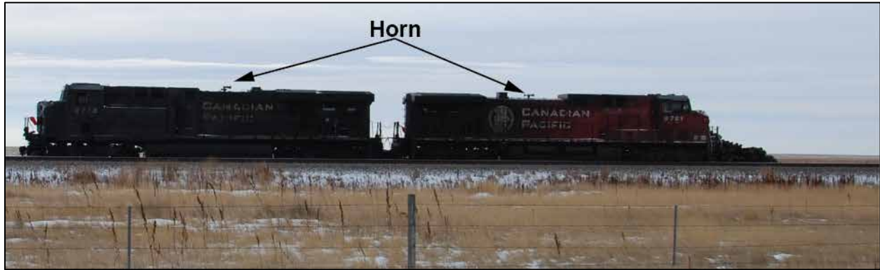
Photo 1. Horn placement on occurrence locomotives
