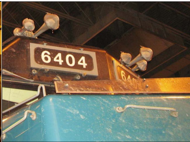
Photo 2. Emergency horn on locomotive VIA 6404
