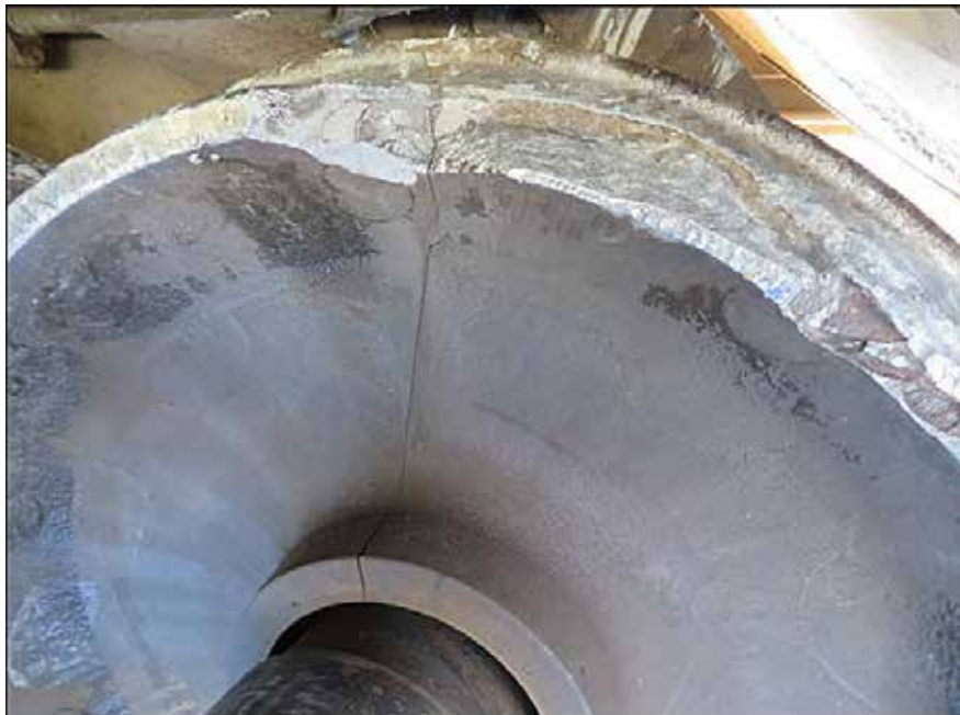
Photo 2. Crack in L3 wheel of car CRDX 15109
