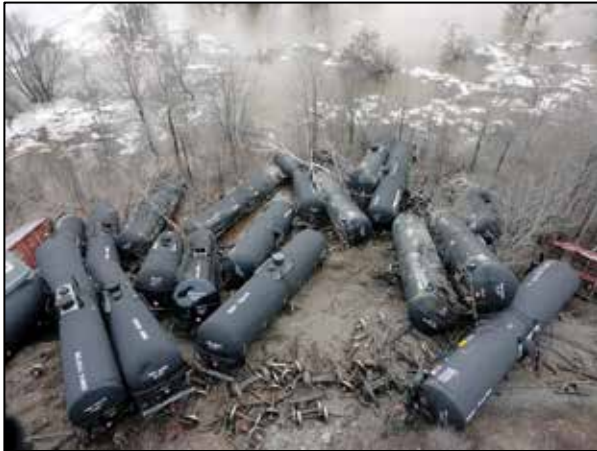
Photo 1. View of the derailed residue tank cars on the embankment toward the Saint John River (Source: Edmundston Fire Department)
