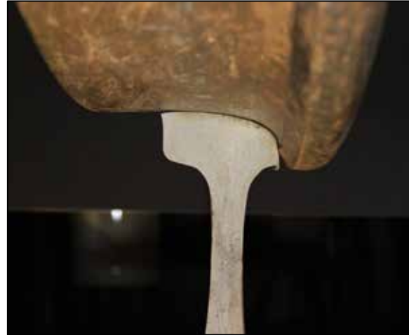
Photo 8. Actual wheel profile of L-1 wheel of the 62nd car compared with contour of high (south) rail. Note: The wheel-rail contact surface has shifted towards the field side of the rail.
