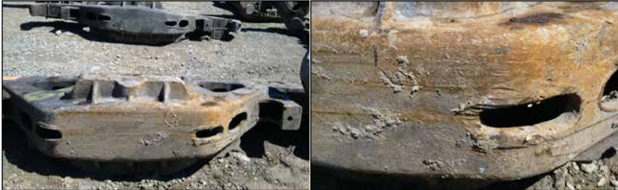
Photo 6. Scratches on bottom of one truck side frame from B-end of the 62nd car
