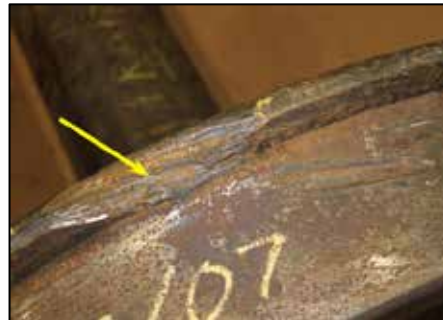
Photo 12. View of mechanical damage on wheel from car DWC 627099
