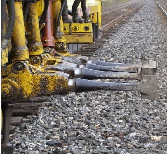
Figure 7. Tamping tools extended (Source: TSB)
