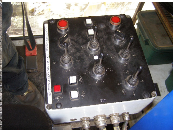
Figure 8. Rotary switches and joysticks in the cab of the tamper (Source: TSB)
