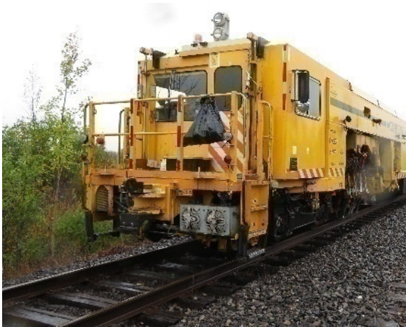
Figure 5. Unimat tamper with long nose leading (Source: TSB)
