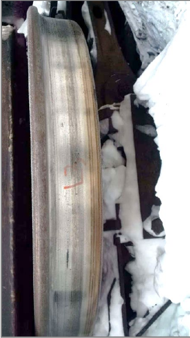
Figure 23. Wheel tread with no blueing (Source: TSB)
