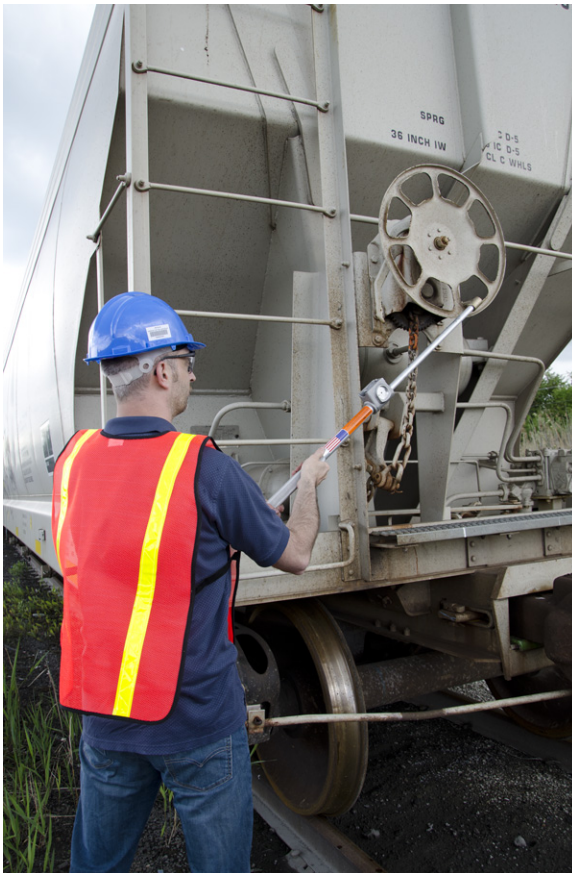
Figure E2. Conductor using a brake stick to apply a hand brake from the ground (Source: Aldon Company, Inc.)
