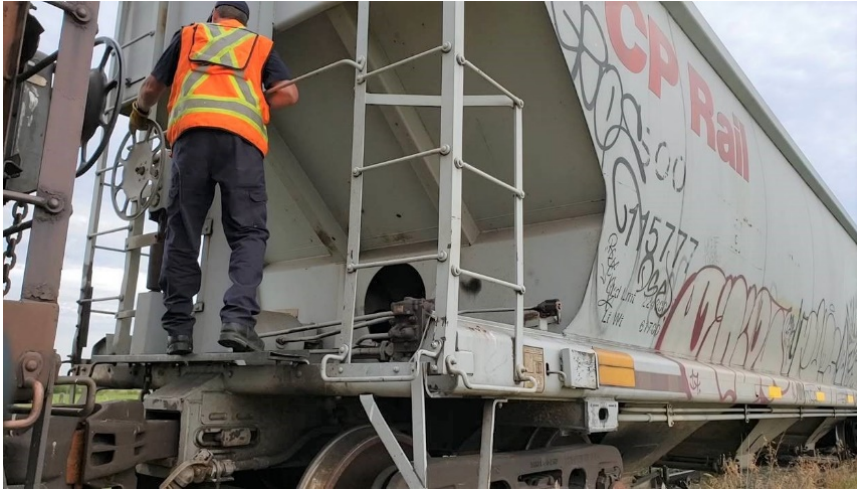
Figure 13. Conductor applying a hand brake (Source: TSB)
