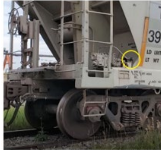
Figure 12. Retainer on a rail car (Source: TSB)
