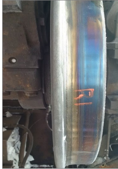
Figure 24. Wheel tread with very heavy blueing (Source: TSB)
