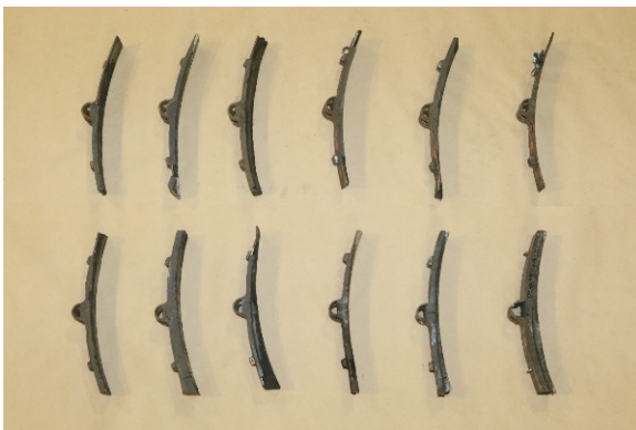
Figure 8. Twelve of the recovered locomotive brake shoes (Source: TSB)
