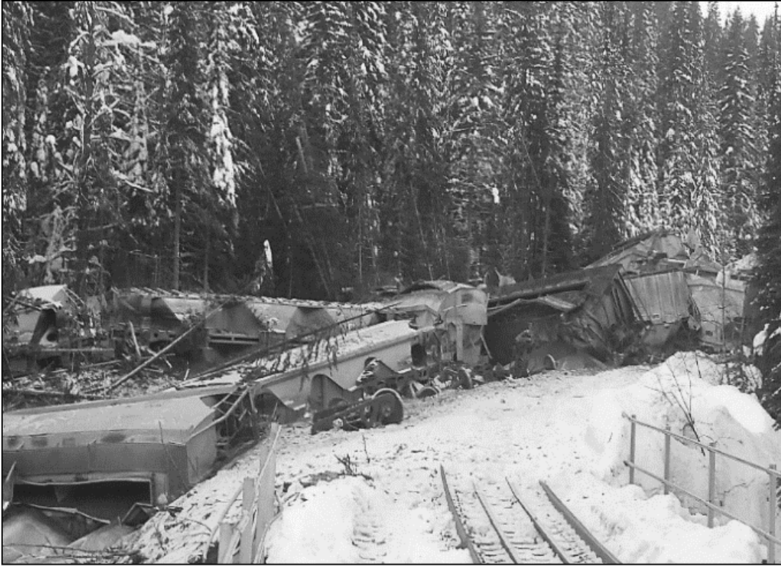
Figure 4. Derailed head-end cars looking toward the rear of the train (Source: Canadian Pacific)
