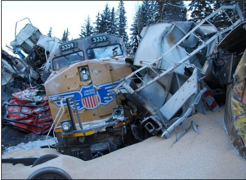
Figure 6. Mid-train distributed power remote locomotive, UP 5359 (Source: TSB)
