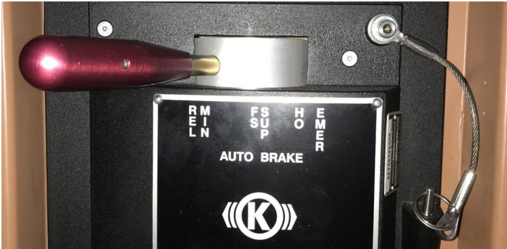
Figure A3. Automatic brake valve handle (Source: Canadian National Railway Company)
