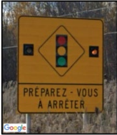
Figure 4. Advance sign installed on Route 116 (Source: Google Maps)
