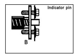
Figure 5 - Indicator Pin in A) Locked Position and B) Unlocked Position
