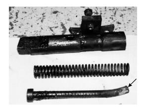
Figure 6 - Bent Lock Indicator Pin
