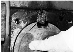
The hitch is designed so that the rotor lock plunger should not self-unlock when the engagement depth of the lock plunger exceeds approximately 1/8 inch.
